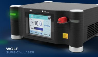
The smallest "CO2 + KTP"-like laser unit for coagulation, vaporisation and bloodless surgery inside an extremely flexible glass fiber.
